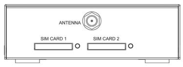
Figure 3 - GWR Router back panel (GPRS and EDGE)
