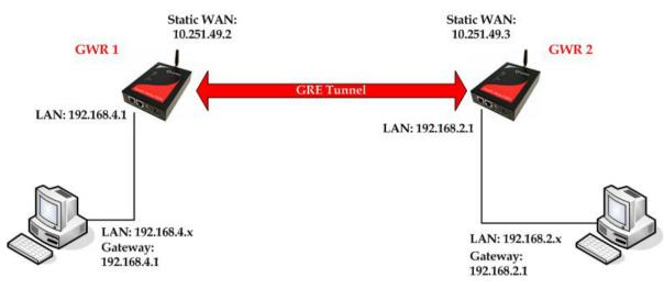
Figure 49 - GRE tunnel between two GWR Routers
