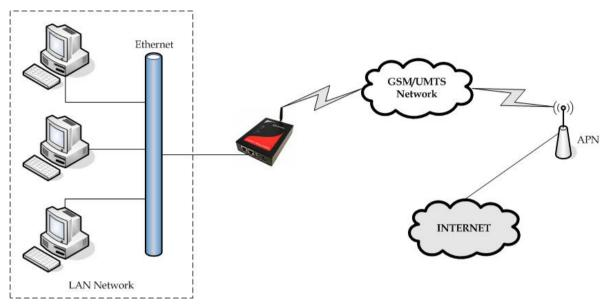
Figure 48 - GWR Router as Internet router
