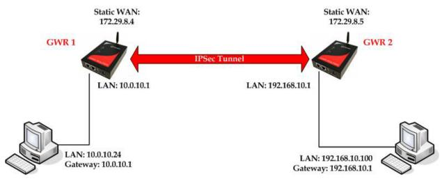
Figure 60 - IPSec tunnel between two GWR Routers
