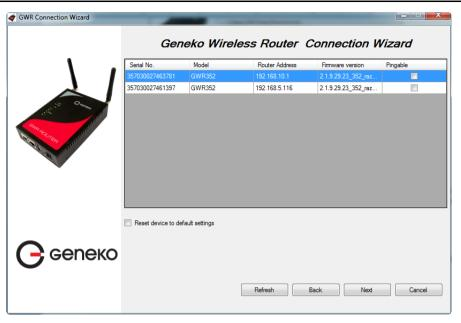
Figure 43 - Connection Wizard - Router Detection
