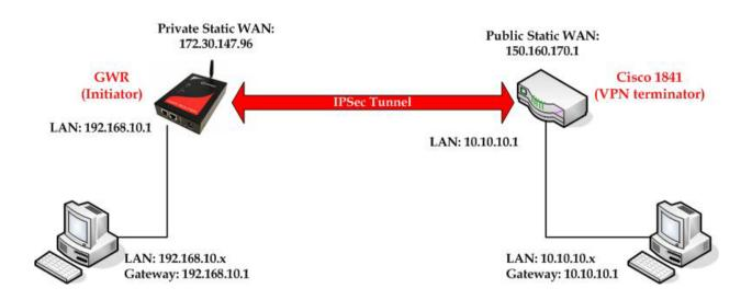
Figure 71 - IPSec tunnel between GWR Router and Cisco Router
